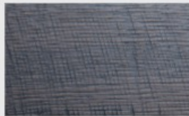
Stained and lacquered mud- coloured oak / chainsaw structure
